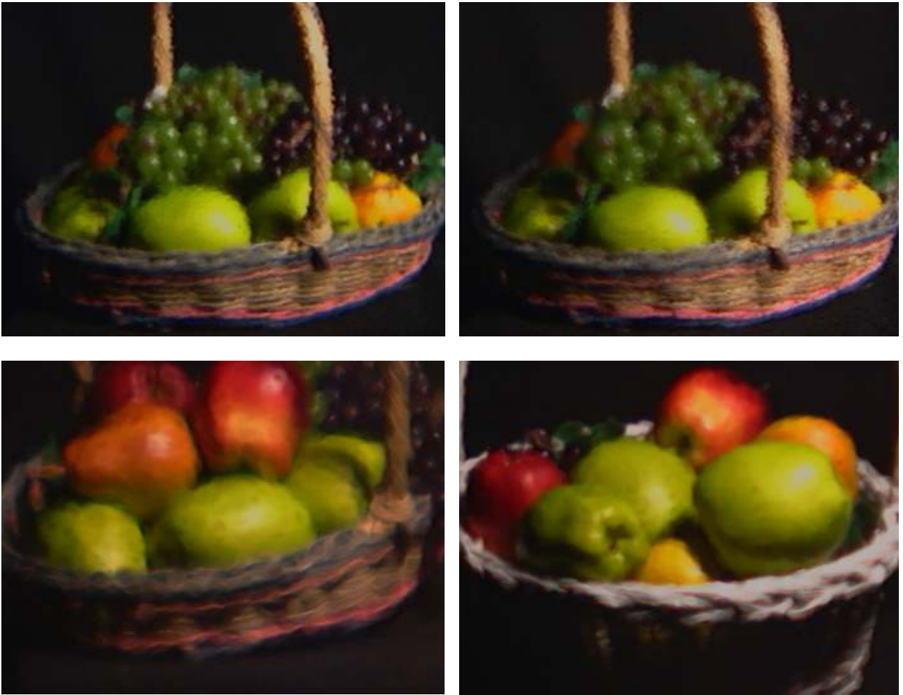
Figure 4.3 Images obtained on the bench setup with: (a) 5mm defocus of the optical phase plate with respect to the intermediate image plane; (b) same as in (a) with some additional defocus introduced by the front objective; (c) closeup view of the scene with the same amount of defocus as in (b); (d) another closeup view of the scene with the same amount of defocus as in (b).
