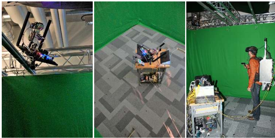
Fig. 17. FWF terminal setup in 4 \times 4 \times 3 meter indoor testing facility at BCOM laboratory. The AP terminal in one corner at 3.5m height (left), the UE terminal on the room floor (centre) and VR-HMD connected to the UE terminal (right).
