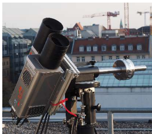
Figure 1. specMACS VNIR and SWIR sensors on the scanning mount. The stray light protection is prominently visible in front of the sensors.
