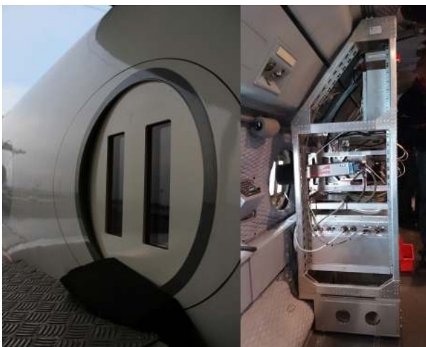
Figure 20. specMACS mounted on the HALO aircraft equipped with the side view port.
