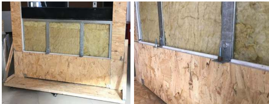
FIGURE 11: Full-scale model and connection details (source: authors' own data).
