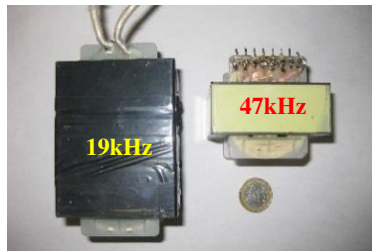
Fig. 6 – Reduction in size of inductor from 3xE65 cores (left) for 19kHz ferrite inductor to 1xE65 core sets for 47kHz KoolM \mu inductor
