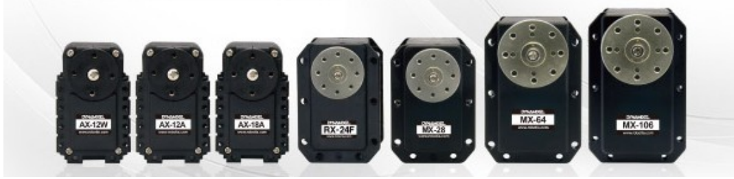
Figure 2.1: DC servo motor products called “Dynamixels” of ROBOTIS (source: [1]).
