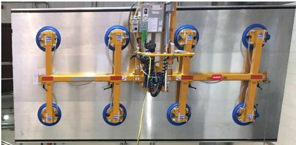
Figure 14: Rigging system used to grip and move CRT modules.
