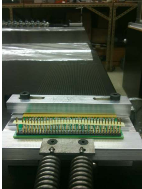
Figure 21. Photograph of a collection plane wire carrier board on the tension stand.
