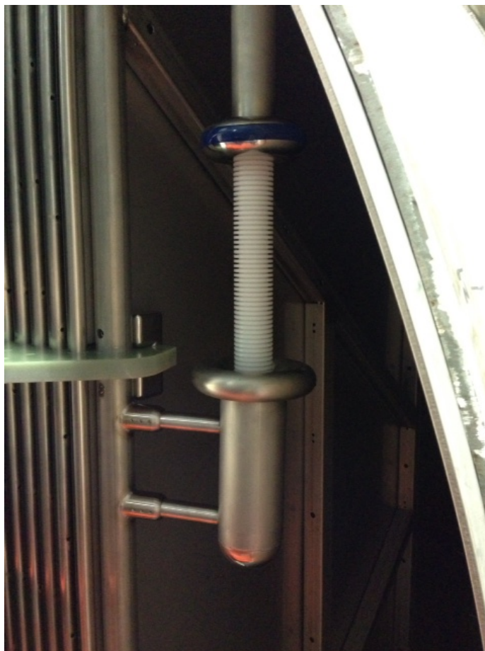
Figure 26. The production HV feedthrough inserted into the cathode receptacle cup inside the cryostat.
