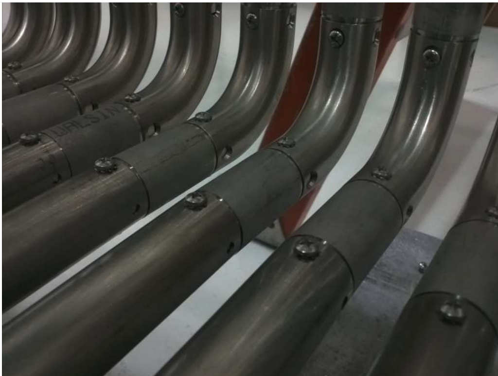
Figure 12. Field cage loop corner, showing elbow and couplings.
