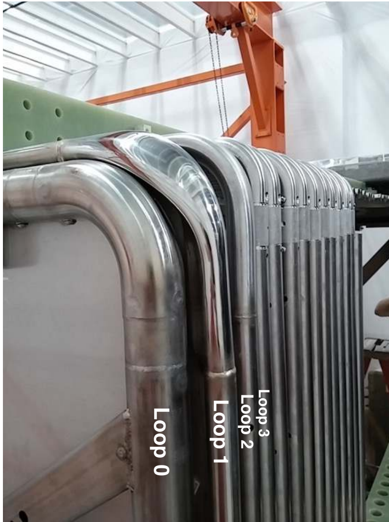
Figure 13. Photograph of the field cage during construction, with loops 0 (cathode) through 3 labeled. Field cage loops closest to (and including) the cathode are modified to reduce sharp edges that would result in higher electric fields.
