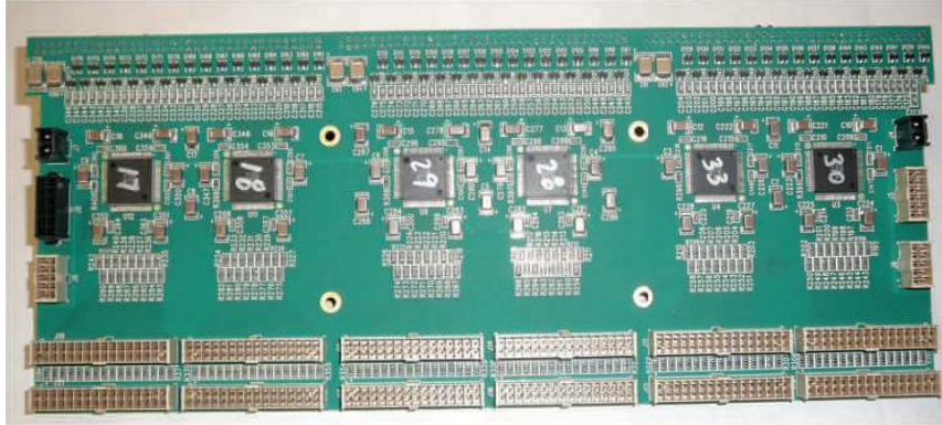
Figure 48. Top version of cold motherboard with 12 ASIC chips, including 6 chips mounted on the top layer and 6 chips on the bottom layer.
