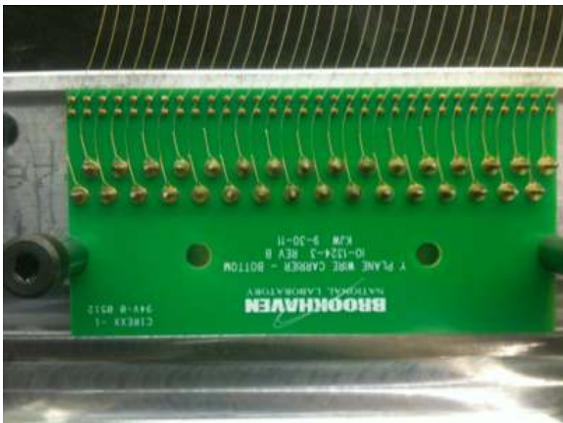
Figure 20. Photograph of a collection plane wire carrier board that has been filled with wires, but has not yet had the cover plate installed.
