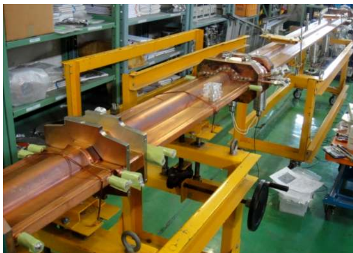
Fig. 8. (Color online) Copper beam pipes for wiggler sections.
