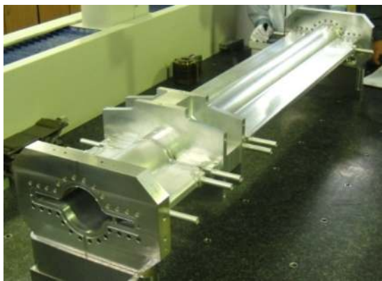
FIG. 9. (Color online) Prototype of an aluminum-alloy beam pipe for the arc sections.
