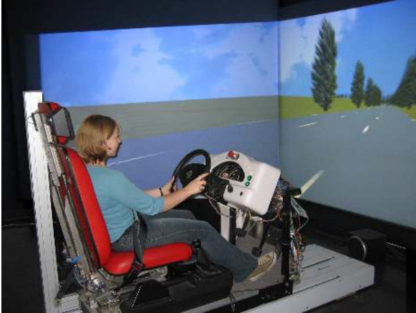
Fig. 17. INRETS/IBISC SIM 2 mini driving simulator: the complete actual set-up in action.
