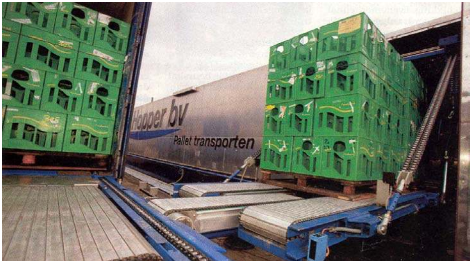
Figure 4.2 Distrivaart: A conveyor-supported automated compact storage system on a barge (source: De Koster and Waals, 2005 ).
