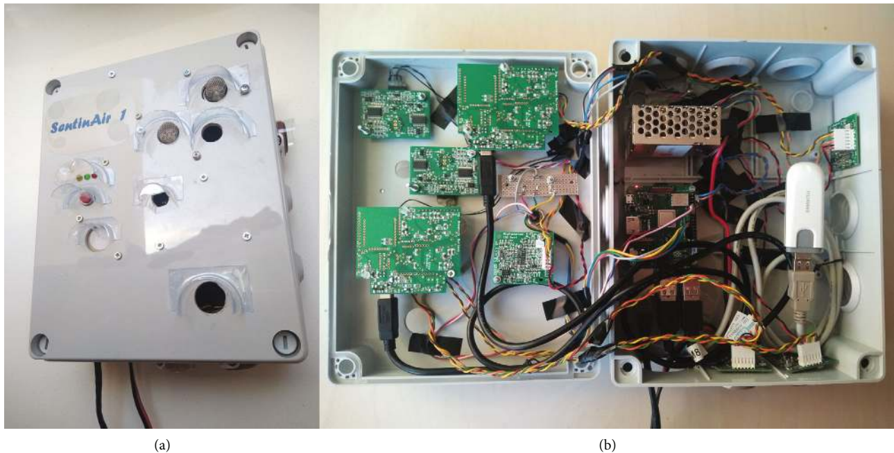
FIGURE 2: SentinAir system prototype. Dimensions are 24, 5 cm x 20 cm x 9 cm. (a) External view. (b) Inside the device with sensors mounted for the second experiment (see Section 3.2).
