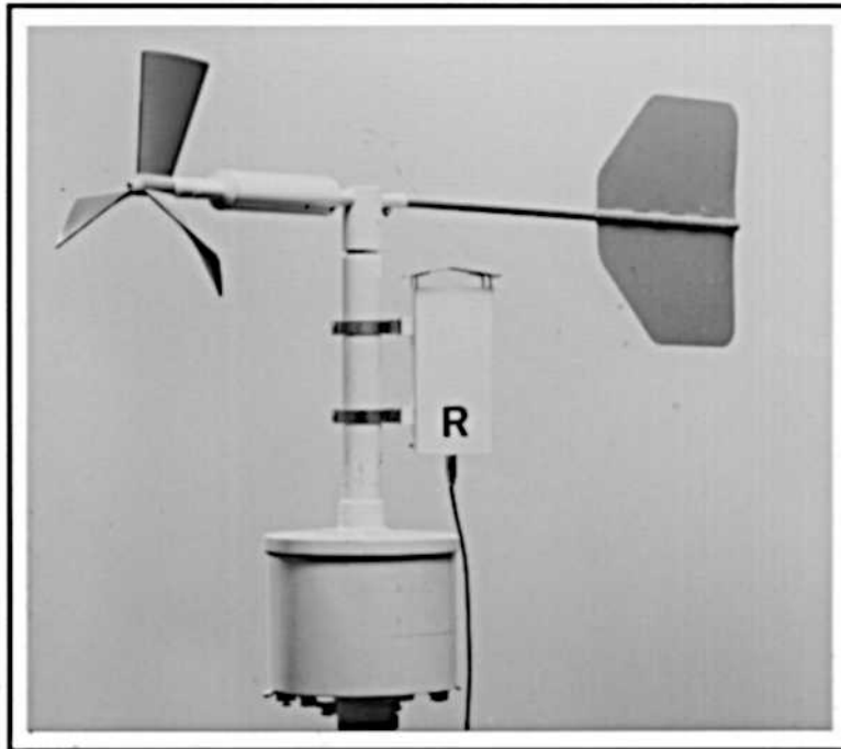
Figure 4.10: The sensors of the weather station.
