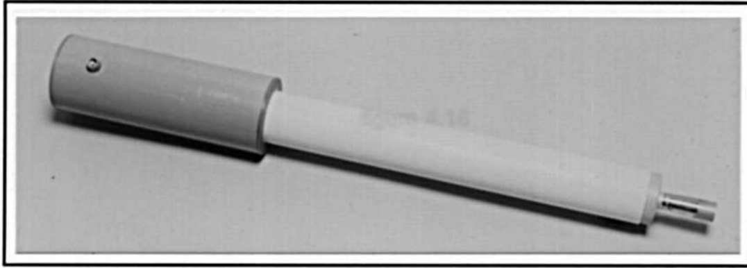
Figure 4.16: The specially developed calibrator for the on-site calibration of the antenna-microphones.
