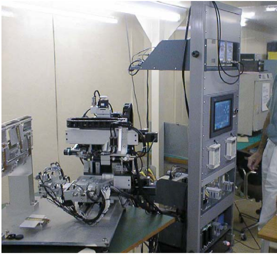
Fig. 4. Picture of the robot together with a simulation barrel stand shown in the left and the control rack in the right.
