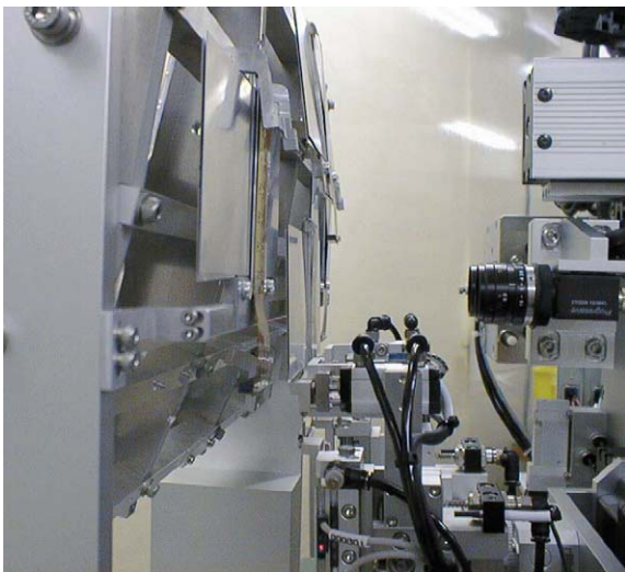
Fig. 5. Close-up of the robot head; the robot holding a module is approaching toward the bracket on the simulation barrel stand.
