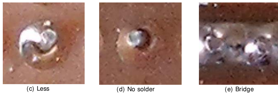
Figure 16: Different types of solder joint appearance
