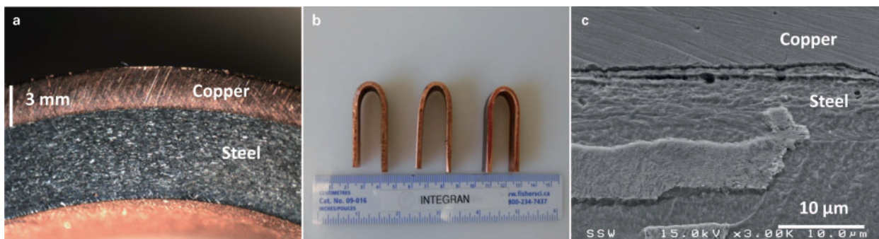
4 Images of electrodeposited sample showing a close up of steel/copper interface (via optical imaging), b results of bend test for 15 cm long, 3 mm thick coating samples heated (from left to right) to 25°C (i.e. as deposited), 60°C and 120°C (via optical imaging) and c etched cross section (via SEM)
