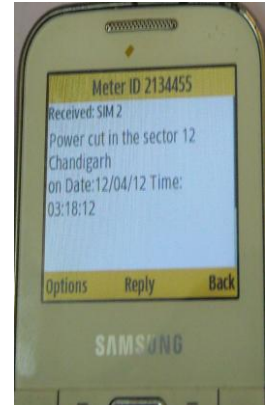
Fig 7: Power cut alert received at energy provider authorized number
