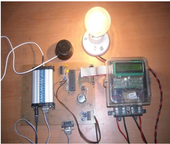
Fig 4: Prototype modal of GSM based energy meter
