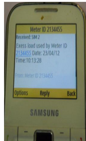
Fig 9: Excess load alert received at energy provider authorized number
