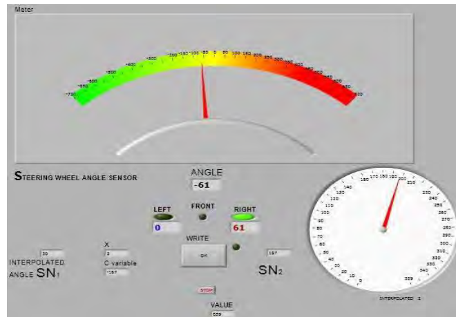
Fig 3 (b) LabVIEW front panel which shows the angle value with steering wheel rotation
