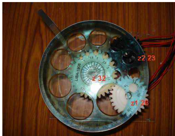
Fig 1. (b) Experimental setup for four circles absolute angular position sensor system ent of a steering wheel angle sensor
