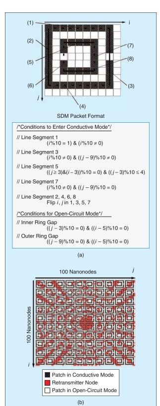
**Figure 6.** Simulated creation of an SRR pattern on a SDM. The directives of the top inset, once relayed and evaluated by all control agents based on their i, j indices, produce the SRR pattern of the bottom inset. A logical "OR" connects the separate conditions.
