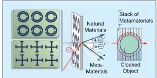
Figure 2. SRRs and crosses are common MM patterns (left). Stacks of carefully designed SRRs can e.g. "cloak" an object (right).
