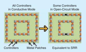
**Figure 4.** SDM controllers act as programmable switches, dynamically "stitching" passive elements into MM patterns.
