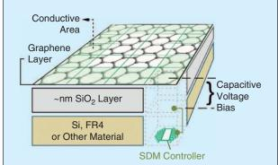
**Figure 5.** A graphene layer can be controlled to become transparent to electromagnetic waves locally, enabling the formation of MM patterns upon them. The SDM controllers form an array of local capacitors with the continuous SiO<sub>2</sub> and graphene layers by regulating their voltage [12].
