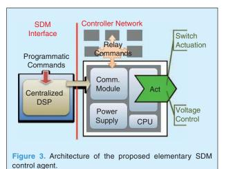
The control agents receive programmatic commands, relay them through their network and act upon the SDM substrate, stitching together typical MM patterns. The origin of the commands can be either internal or external to the SDM. In the former case, a standard computer can interface and interact with the SDM, while in the latter we assume that the control agents can operate more autonomously. For instance, they could sense their environment and react automatically in an collaborative fashion.
