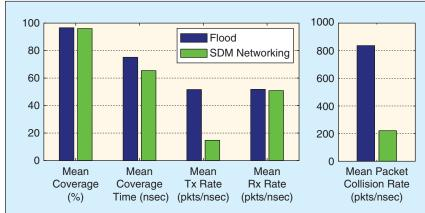
Figure 7. SDM-tailored networking yields high reachability, lower energy expenditure and improved SDM programming speed (coverage time) than a flood-based approach.
