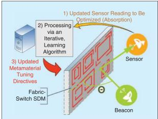
Figure 8. A potential SDM application scenario, featuring an angle-independent electromagnetic absorber, accentuating the SDM programmability, interconnectivity, and adaptivity potential.
