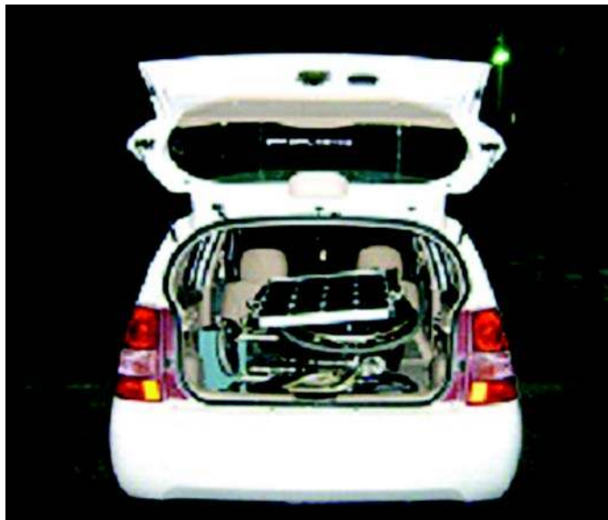
Figure 9. Photograph of folded prototype wheelchair in car trunk.
