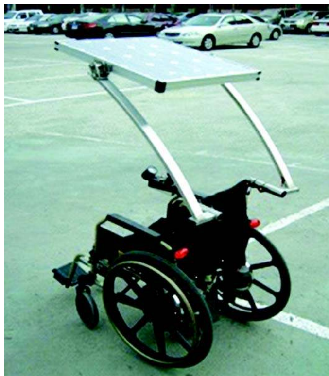
Figure 3. Photograph of prototype of solar power-assisted manual/electric wheelchair.
