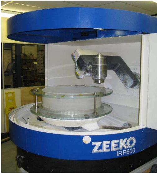
Fig. 13: Thin shell mounted on the IRP600 polishing machine at the Zeeko facility. The SSS supplies the suitable interface to the machine, keeping the shell at the right vertical position necessary for the polishing.
