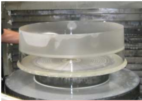
Fig. 8: Raw quartzglass tube mounted on the grinding machine at the Heraeus Quarzglas facility.
