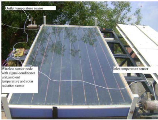
Fig.2. Flat-plate collector with sensor node mounted on it.
