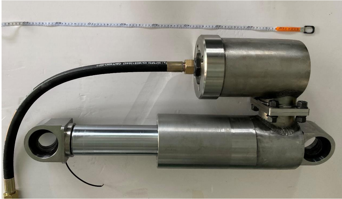
Figure 19. The prototype of the MR hydro-pneumatic spring damping structure
