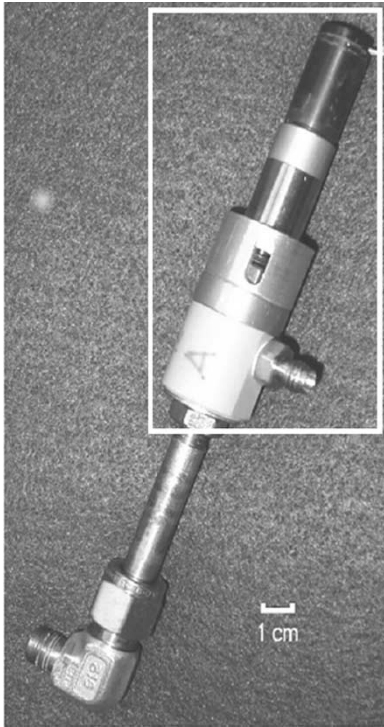
Fig. 1. Prototype proportional liquid fuel valve (shown in box), with the catalyst pack attached at the output.
