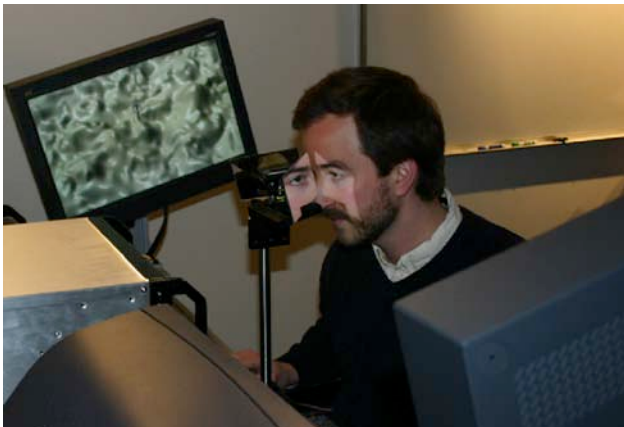
Figure 6. A retinal resolution digital stereoscope used for evaluating visualization methods.
