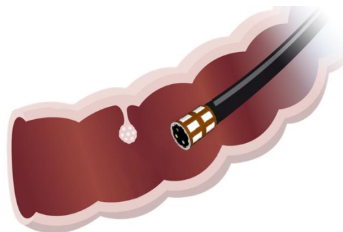
Fig. 1. Diagram of the proposed MI system for colonoscopy including the antenna applicator attached at the tip of a conventional colonoscope.
