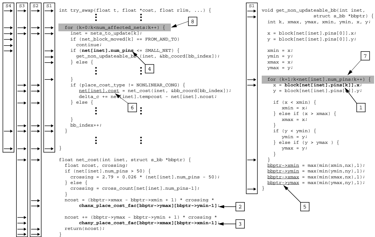
Figure 3: VPR code example. Labels “1”-“4” indicate cache-missing memory references selected for slicing. Labels “5” and “6” indicate memory references requiring store removal. Labels “7” and “8” indicate loops that bound the scope of slicing. Labels “S1,” “S2,” “S3,” and “S4” show the slice result for the selected memory references.
