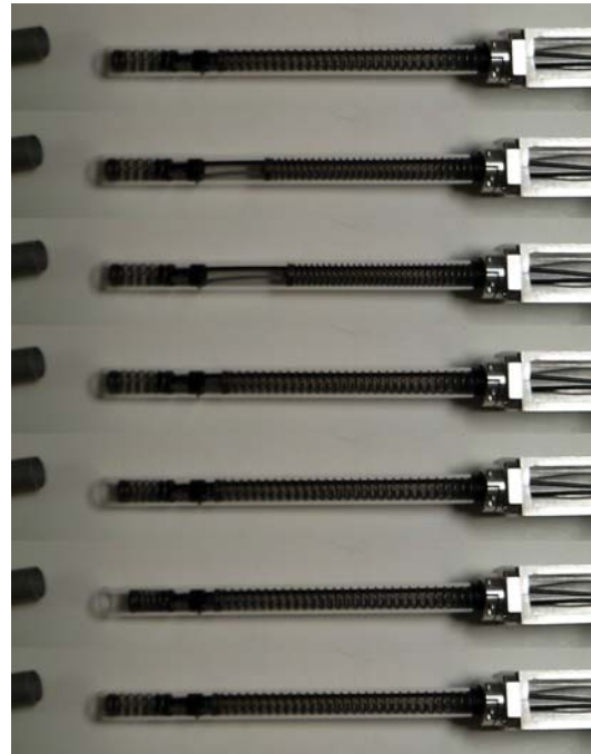
Fig. 5. Behavior of the inner tube compression spring design of an end cap. External cables attached to other end caps run into the tube and attach to one of two springs. Each spring is fitted with a custom compression sensor for spring tension sensing independent of the angle of the external cable. The whole assembly slides into an aluminum tube, allowing for various configurations and strut lengths.
