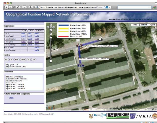
FIGURE 10: AnaVANET replaying a VANET experiment. Buildings avoid a direct line-of-sight communication, thus forcing the usage of multihop routes.
