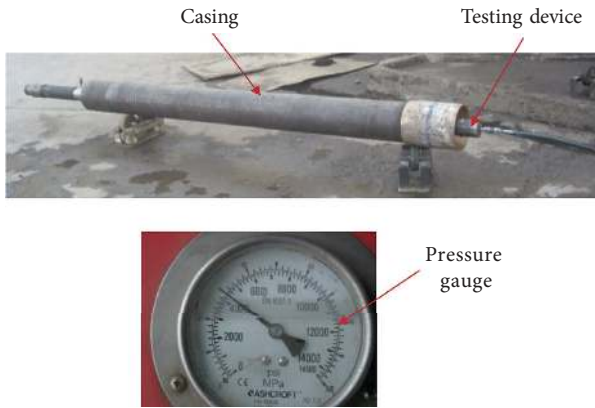
FIGURE 24: Pressure testing device and pressure gauge.
