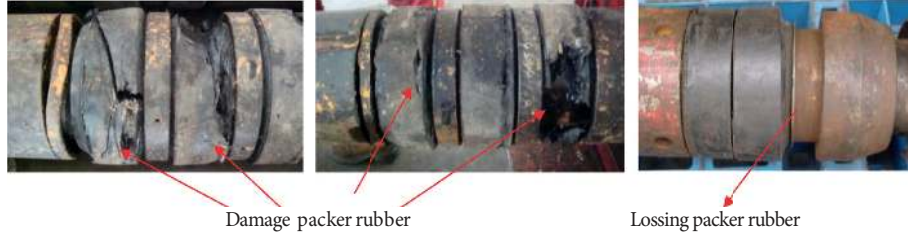
FIGURE 2: Failure cases of the rubber packer.
