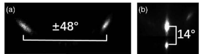
Fig. 16. (a) Scanning range in \Phi axis. (b) Scanning range in \theta axis. See Visualization 2 for video showing the 2D scanning tested by the scanning test system.
