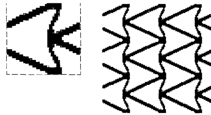
Figure 3. Material with Poisson's ratio -0.8 obtained from a ground structure with 40 by 40 elements and vertical symmetry enforcement.
