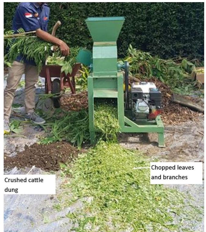
Figure 7: The machine in action
