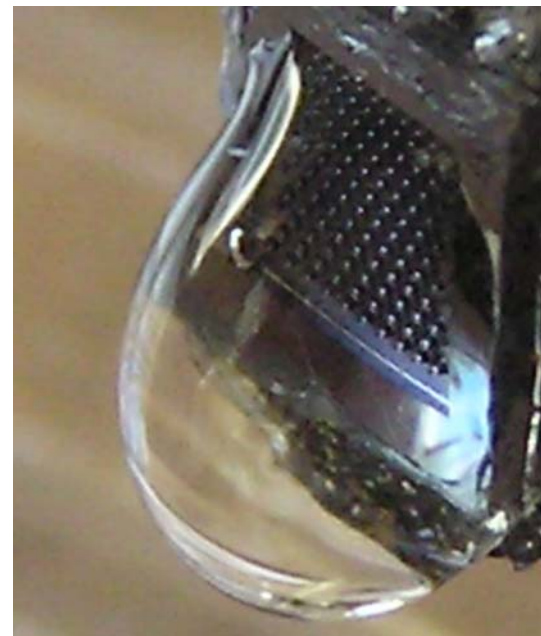
Fig. 4 Delivery test, showing a droplet formed on the end of the array
