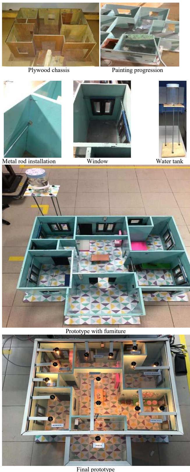
FIGURE 4. SH prototype fabrication.
