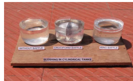
Fig. 8 Experimental Setup to Demonstrate Slosh & Damping
