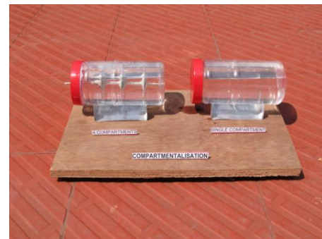
Fig 12: Experimental Setup to Demonstrate Compartmentalisation to Reduce Slosh
