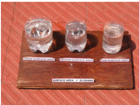
Fig 10: Experimental Setup to Demonstrate Sloshing vs. Surface Area
