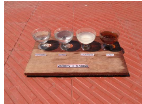
Fig 11: Experimental Setup to Demonstrate Sloshing vs. Viscosity of Liquids
