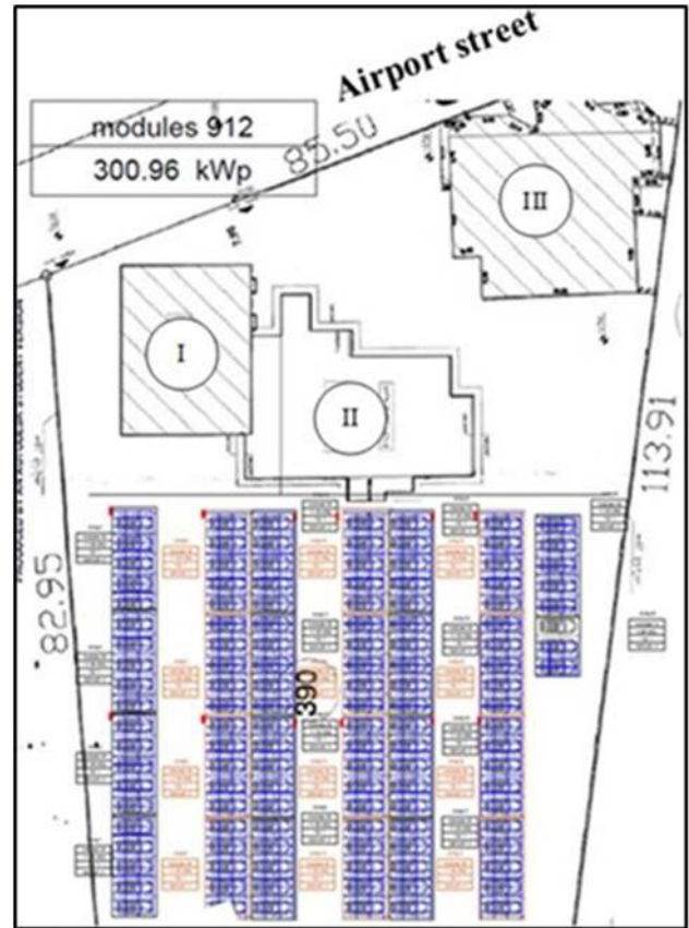
Fig. 15 Modified parking plan with PV panels
