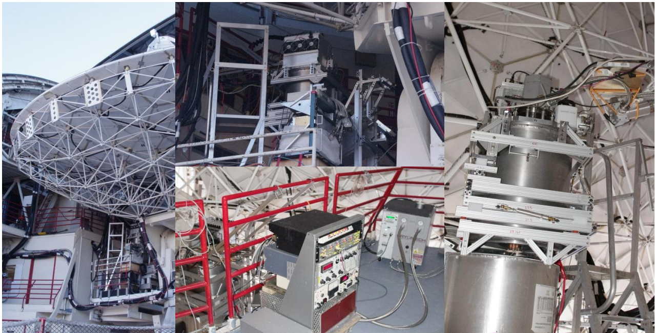
Figure 11: (left) ZEUS-2 on the nasmyth-2 platform at the CSO. (middle top) ZEUS-2 on the nasmyth-2 platform clearing showing the MCE with three cooling fans, and fore-optics. (right) ZEUS-2 and mount at the CSO. (middle bottom) ZEUS-2 electronics rack and pulse-tube compressor at the CSO. ZEUS-2 is beyond the red railing on the left.
