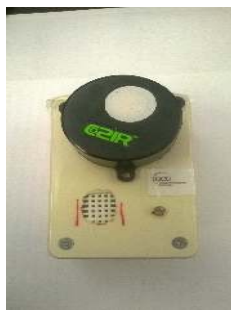
Fig. 3. Environment Monitoring Sensor Node. Algorithm for Occupancy Estimation using Door Sensor Node, RNN Occupancy Estimator and Hybrid RNN Occupancy Estimator are embedded in Environment Monitoring Sensor Node
