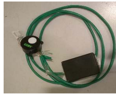
Fig. 4. HVAC duct Sensor Node
