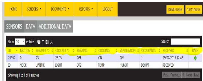
Fig. 20. View of Webportal- Control Parameters of HVAC from Smart Controller and Occupancy Estimation are displayed by clicking on More Button of Main Page.
