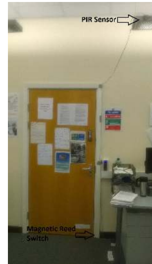
Fig. 5. Door Sensor Node, PIR sensor Node for detecting the movement and magnetic reed switch to detect the door opening/closing
