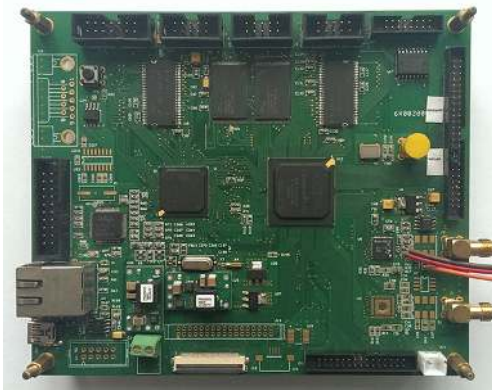
Fig. 11. Photograph of the signal processing board.
