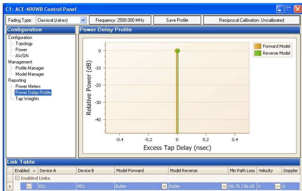
Figure 8.2: Power delay profile of the ITU-T Butler model
