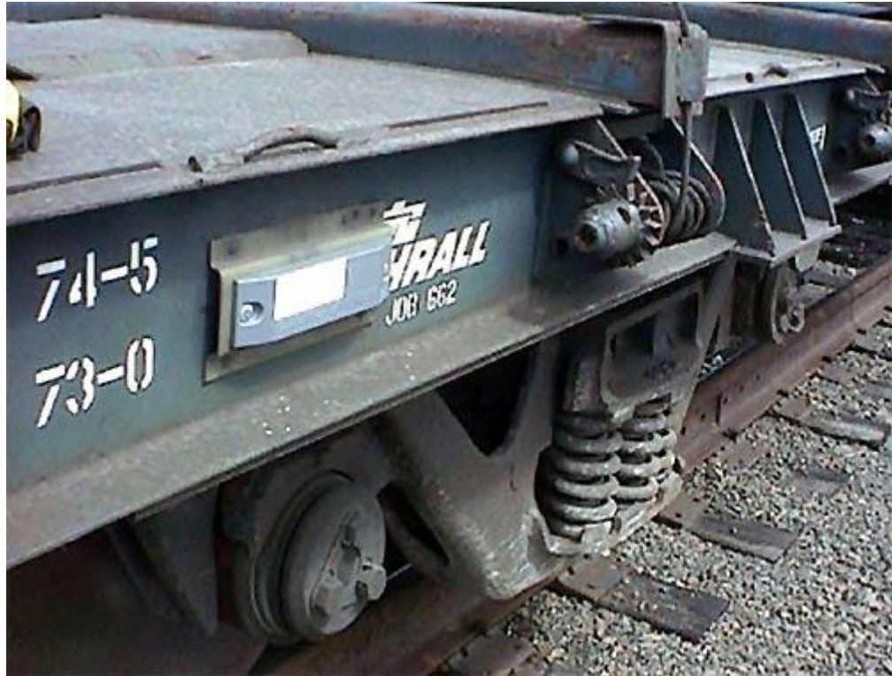
Figure 1.4: A railcar with an AEI tag mounted on its side [7]
