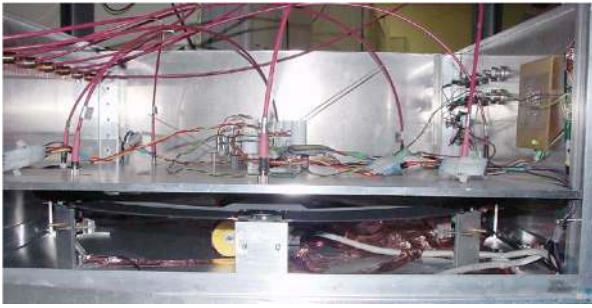
Fig. 2 The detection unit. The PMTs and the detector fibers were arranged in a circular geometry and fixed. A rotation stage was used to change the positions of the filters.
