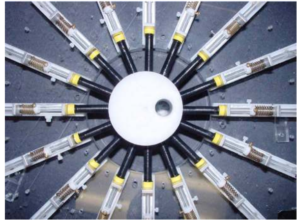
Fig. 3 The fiber optic adaptive interface, fiber optic probes, and the solid phantom with a hole.
