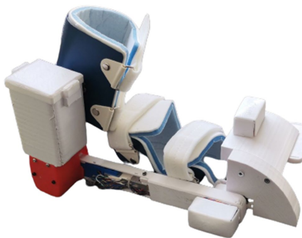
Fig. 5 Isometric view of the 3 DoF proposed exoskeleton
