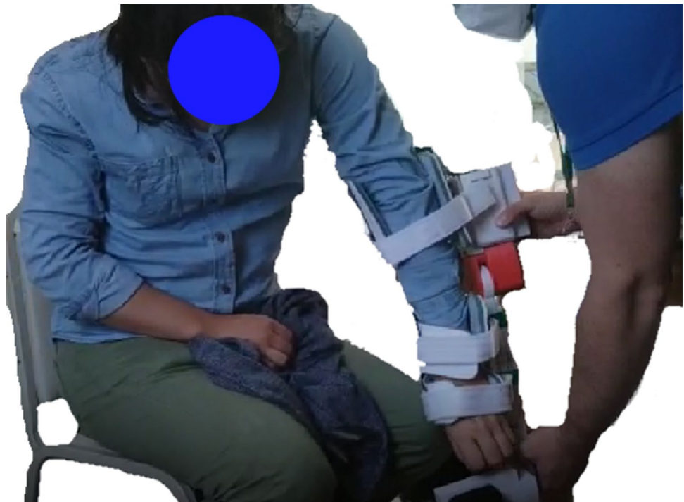
Fig. 8 The placement of the proposed exoskeleton on a user is simple. Velcro bands are unfastened from the orthosis attached to the mechanical system. Then the user inserts the arm over the system aligning the joints. Finally, the velcro bands are adjusted
