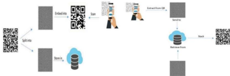
Fig. 5. (left) Construction of VCS and(right) Stacking of vcs.
