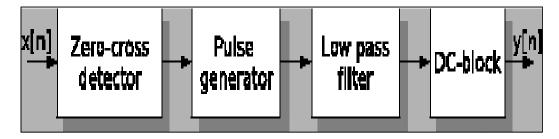
Fig. 7. Zero crossing detector
