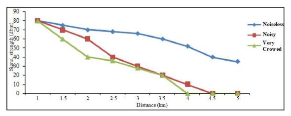
Fig. 16. Distance vs signal strength analysis for different noise levels
