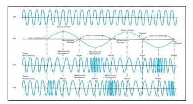
Fig. 1. The FM signal generation
