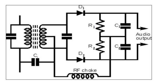
Fig. 8. Foster-seeley FM detector circuit
