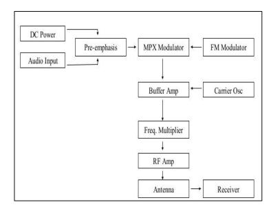
Fig. 9. Flow diagram of the FM transmitter operating principle
