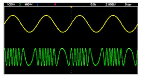
Fig. 14. The FM modulated signal (green) and message signal (yellow) using digital oscilloscope (simulation output)
