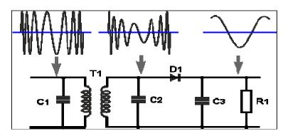
Fig. 6. Circuit diagram of slope detector
