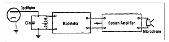
Fig. 3. The direct method of FM generation circuit
