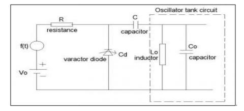
Fig. 4. Varactor diode FM modulator
