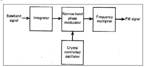
Fig. 5. Indirect method of generation
