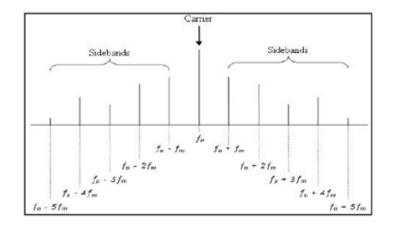
Fig. 2. The FM frequency spectrum
