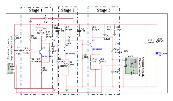
Fig. 10. Circuit diagram of wireless FM transmitter realised using multisim simulator
