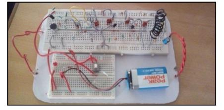
Fig. 11. The FM transmitter circuit that is designed
