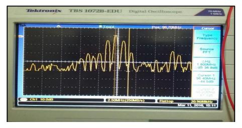
Fig. 15. The FM output captured using frequency analyzer (tuned at center frequency of practical test case)
