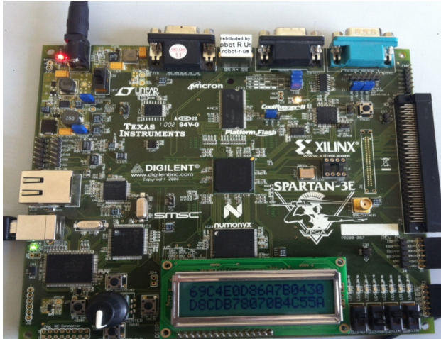
Fig 6.1 Snap Shot of Cipher Key, Plain text, recovered plain text, recovery key on FPGA
