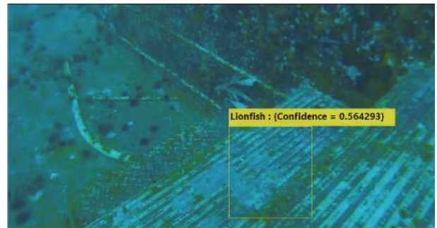
FIGURE 11: An example of false positive detection due to similarity of patterns. Although because of strip patterns this stair was detected as a red lionfish, the confidence was about 0.5 that is below the defined rejection threshold. Location of image is TDC Reef #1.
