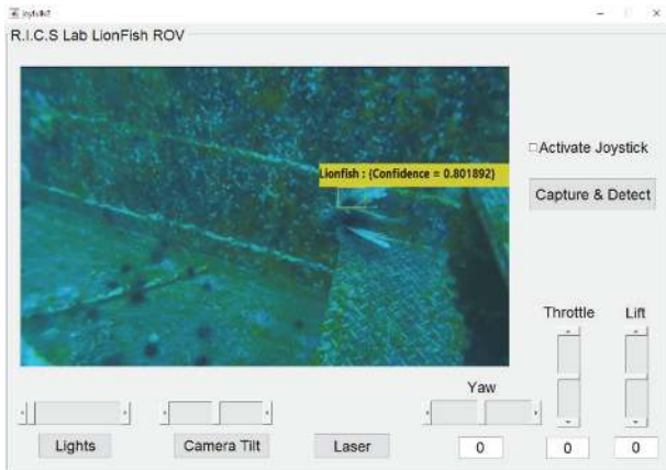
FIGURE 6: Designed UIP in MATLAB. All three brushless motors, LED lights, camera, laser, and camera tilt are accessible via this UIP. Live camera view also is available on this UIP.
