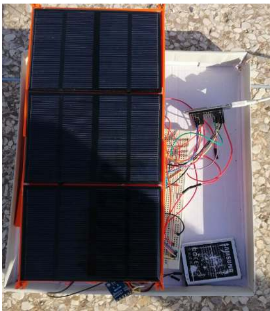
Fig. 10 PV panels under shading effect
