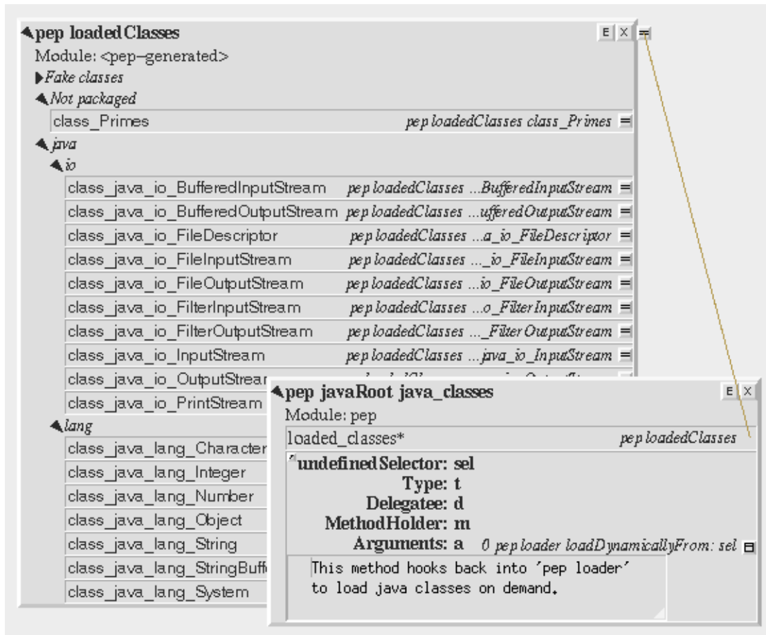
Fig. 18. Lazy class loading implemented by catching message-not-understood errors.
