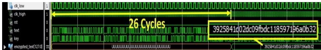
Figure 15. The ISim simulation of the normal AES processing
