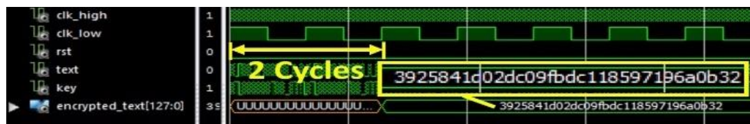
Figure 17. The ISim simulation of the parallel AES processing
